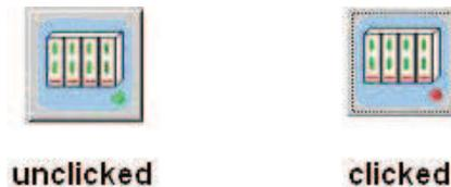
Click on the drivers such that the LED turns red and the drivers are thus engaged. With the drives engaged, the brake should be disabled. If the drivers are disabled, the brake should be enabled.
