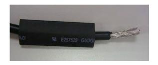
(1) Cut through the cable and expose the core wire which covers the metal core wires with shielding. The reserved core wire length should be 20~30mm. Then, cover a 45mm heat shrink tube on the cable.
