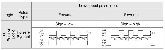
For digital circuit, it uses 0 and 1 represents two status, which is high voltage and low voltage. In Positive Logic, 1 represents high voltage and 0 represents low voltage and vice versa in Negative Logic.
