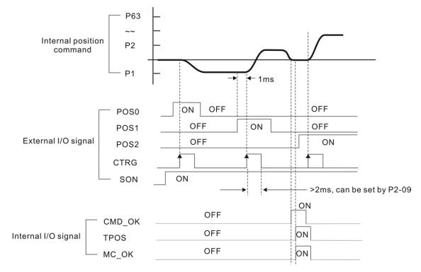
$\mbox{CMD\_OK}$  :  $\mbox{CMD\_OK}$  is activated when the servo drive has detected that  $\mbox{Pr}$  command has been completed
