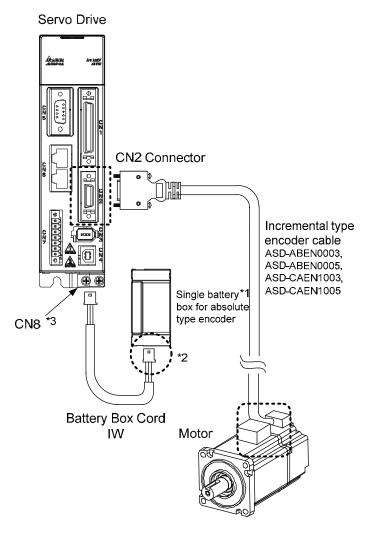
This is the wiring diagram for connecting to a single battery box. The scale of the objects does not match the dimensions as shown in the drawing above. For different models of AC servo drives and motors, the connection cables may differ.
