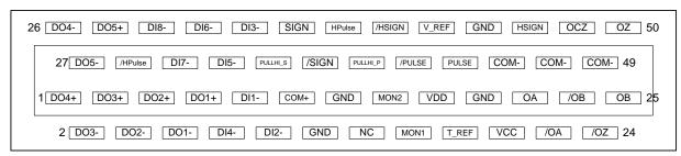
The rear wiring terminal of CN1 connector
