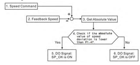
1. Speed command: It is the command issued by the user (without acceleration / deceleration), not the one of front end speed circuit.
