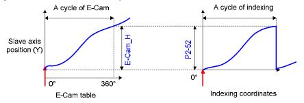
Note 1: ECAM\_H (height of E-Cam table) = E-Cam table (last point - first points)
