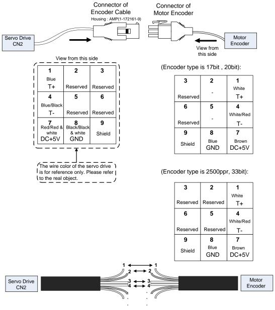
If not using housing and directly wire the cores, please follow the corresponding core number for wiring. For example, core number 1 from the servo drive CN2 should connect to core number 1 from the motor encoder; core number 2 from the servo drive CN2 should connect to core number 2 from the motor encoder and so on. Please number the cores from the servo drive in order and then connect it to the encoder.
