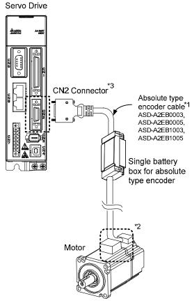
This is the wiring diagram for connecting to a single battery box. The scale of the objects does not match the dimensions as shown in the drawing above. For different models of AC servo drives and motors, the connection cables may differ.
