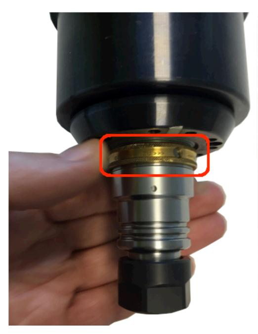
Final step is to close the cover over the hole of the allen key, so no dirt or chips get in there.
