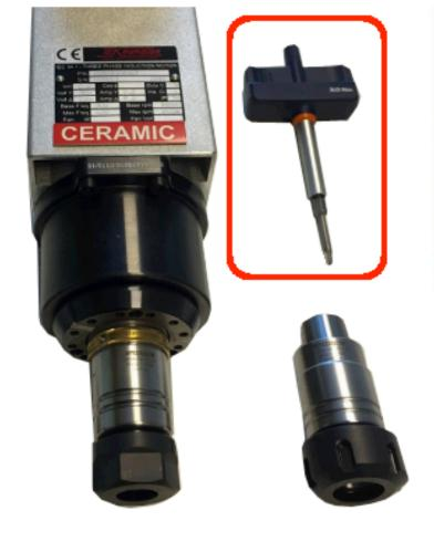
Torquewrench preset to the correct torque is included in the delivery.
