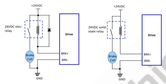
Figure 5: Brake Output Connection
