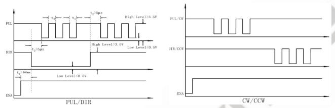
Figure 8: Sequence chart of control signals
