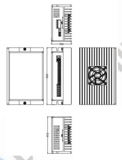
Figure 1: Mechanical specifications
