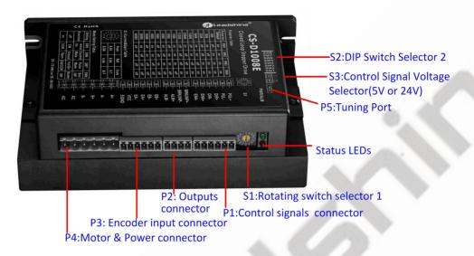
Figure 2: CS-D1008E connectors
