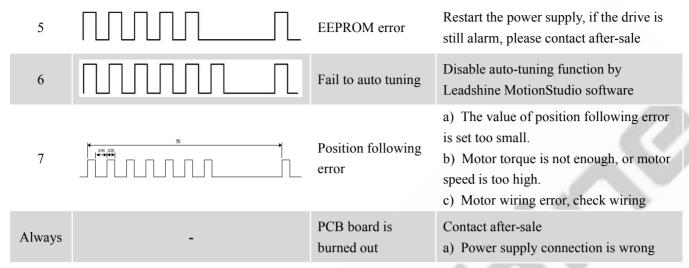
When above protections are active, the motor shaft will be free or the red LED blinks. Reset the drive by repowering it to make it function properly after removing above problems.
