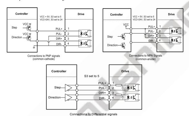
Figure 3: Control Signals Connection
