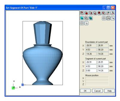
The dialog shows a new drawing of your part, with a rectangle that indicates the (sub)segment that you are editing. The buttons on the right can be used to influence the drawing. Eleven of these are standard DeskProto buttons of which the use is known, and that need no explanation here. Note that mouse rotation is not present: this dialog only used the six main views.
