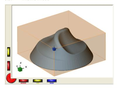
The view window shows the geometry that you are working with. You can have different representations of the geometry in your scene, for instance the original geometry drawn in lines, or the calculated toolpath. Which of these representations is shown can be defined with the Subjects in View dialog. Here you also can select other subjects, like title, orientator and working area.
