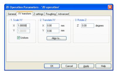
The Transform parameters for 2D are meant to correctly position the 2D plot data over the 3D geometry.
