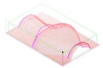
Most lines are drawn as solid lines (default in red), indicating a normal speed (Feedrate). Some are dashed in grey, indicating that they are **Rapid** movements (moving as fast as possible). The toolpath depends on the settings made in the Operation Parameters dialog.
