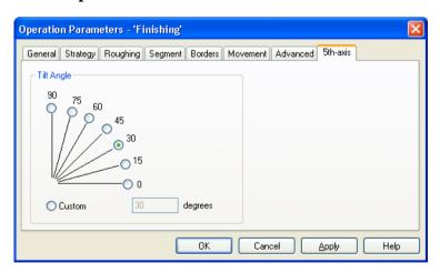
A **5th Axis** is supported by DeskProto only in a special case: the manually controlled B-axis as present on some small wax milling machines for jewelers. Like on the Roland JWX-10 "Jewela" machine, as shown in the illustration below:
