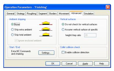
Ambient skipping concerns the ambient area. Basically DeskProto always machines a complete rectangular area (the segment), due to its parallel
