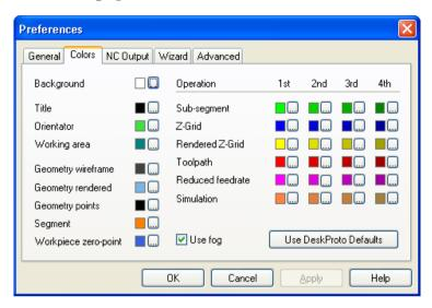
The tab page Colors makes it possible to customize all colors used on the DeskProto screen: just use a [...] button to change any color shown. As you can see different operations can be assigned different colors. In case of many operations: the color for operation No. 1 will also be used for No. 5, 9, 13 etc etc.
