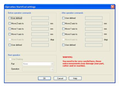
Up to six **Before Operation commands** (or Start commands) can be specified. These will be written as extra lines in the NC program file, just before the toolpath of this operation starts. Each line is optional, and will only be written when checked (checking none will mean that no in-between lines are inserted):
