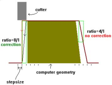
Note that this vertical surfaces check does not work for conical cutters as the steepness of the toolpath is analyzed (for conical cutters the toolpath never can be steeper than the Angle of the cutter). Still checking this option will be effective then: the cutter definition will be changed. The height/step ratio is not used for conical cutters.
