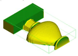
The example drawing above of a Bottle Toolpath clearly shows the rest material in-between the ballnose toolpaths (such ridge is called cusp). In the example the Simulation calculation is interrupted halfway by pressing the button Show Results Now in the Simulation calculation's progress bar. You can exactly see how far the cutter has come.
