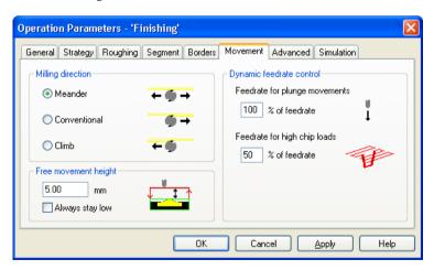
The **Milling direction** is important for the surface quality of the prototype. The default direction is **Meander**, which means that the first movement is from left to right, the second from right to left, etc. The tool keeps cutting all the time, so meander is the fastest option.
