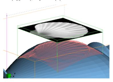
Here a shell relief is created from a bitmap image, and projected on the perfume bottle that you have seen more often as example part. This is of course a great design tool to create embossed products. The picture shows a positive relief: on top of the geometry.
