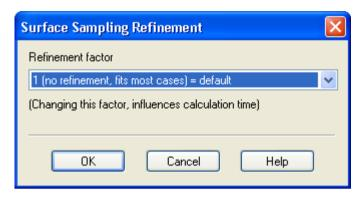
The Surface Sampling Refinement dialog allows you to fine-tune the gridsize or calculation precision. The higher the Refinement Factor, the more accurate the toolpaths and the longer the calculation time (quadratic). A refinement factor 1 will result in a Z-grid with a gridsize that equals the settings for Distance between toolpaths and Stepsize along toolpath. A **Factor 2** will double the Z-grid resolution for both X and Y, so will subdivide each gridcell into 4 smaller cells, etc.
