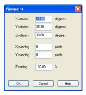
In this dialog you can change the point of view from which you look at the geometry, z-grid, toolpath etc. You can set the values exactly, using the keyboard. The rotations are executed in the order X, Y, Z. The effect is the same as when using mouse rotation, pan and zoom or when using the thumbwheels
