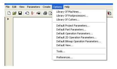
The Options menu gives access to all configuration options of DeskProto. For normal use you will not need these options, they are present in case the defaults set by the installation program should not match your wishes. The option used most will be the creation of a new cutter definition, as the default cutters will not match your real cutters.
