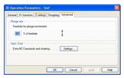
Most of the Movement parameters and Advanced parameters of the 3D Operation do not apply for 2D, only these two settings are useful. The meaning of each setting is the same as in a 3D Operation, so please read that help information:
