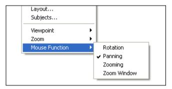
This command determines the functionality offered by the left mouse button inside the View Window. Four different functions are possible, of which always exactly one is active (the four functions are toggled). In the Toolbar you can quickly see which function is active as that button is drawn depressed.
