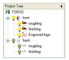
In DeskProto the **structure** of the Project is shown in the project tree, which is placed on the left of the screen. In the above example the project 'Torso' contains two parts, one with three operations and one with two. Two different Operation types are present: the (standard) Operation which is 3D, and the 2D Operation (note the different icon in the Tree).
