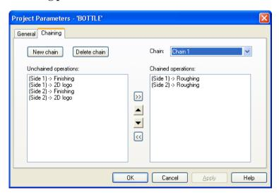
Chaining is an option meant to combine Operations in different Parts into
