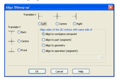
This dialog is used for 2D Operations and Bitmap Operations, and can be reached using the "Align to..." button in the 2D Operation parameters and the Bitmap Settings. As these types of Operations both use their own geometry file, it may be needed to align this geometry with the 3D Geometry as defined by the Part. This dialog makes such alignment easier.
