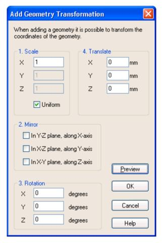
It offers basically the same transformations as also present in the Part Parameters (see there for more help), however these will be applied to the new geometry file only. After adding the second geometry file DeskProto only sees one resulting geometry, making it impossible to later translate or rotate only the new geometry elements.
