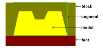
Note: in case Inverse milling (male to female) is applied, then the segments boundaries entered here are applied on the original geometry, before the male to female conversion.
