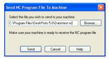
In DeskProto the NC program file must be saved first; a drawn toolpath is not sufficient to use this option. A dialog as shown above will be displayed to ask you for the file you want to transfer. After selecting the correct NC program file and pressing Send DeskProto will start sending. In order to send the current toolpaths without first saving an NC file you can use the command Send current toolpaths to machine.
