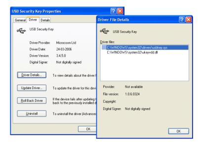
The Driver Tab and Driver File Details dialog show which driver file has been installed. If it does not match the above illustrations (Provider needs to be Microcosm), then you have an incorrect driver installed. Strange is that the Driver File Details dialog not always shows the Provider.
