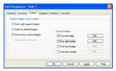
Support blocks or bridges can be added to the geometry to facilitate machining a model from several sides. These are small blocks of material (cylinder or rectangular), acting as connection bridges to hold the model in place within a frame (that has to be larger than the model). Each support block is created using triangles: these will be added to the geometry, and will be handled by DeskProto just like any other geometry detail.
