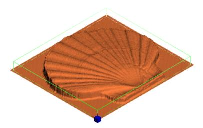
The two pictures above show the original bitmap image of a shell left, and right a simulation of the resulting 3D Relief. Min Z has been assigned to black, and Max Z to white. DeskProto does not display the resulting Bitmap geometry, you can only see it by displaying the Z-grid, the Toolpaths or the Simulation.
