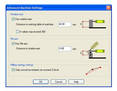
The option to indicate the presence of a **Rotation axis** has to be checked in order to make rotation axis machining available for this machine. If not, the option "Use rotation-axis" in the Part parameters will be grayed out.
