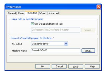
These preferences are meant to configure the NC-output, so the exporting of NC files by DeskProto.
