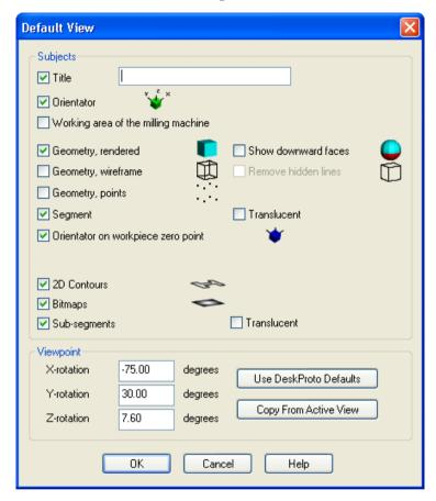
The default view settings are used for any new project and any new part. They are also used for the command and button Use Default View.
