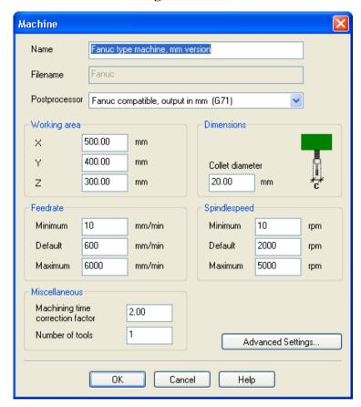
The **Name** is the name that will appear in any DeskProto dialog for selecting a machine. It needs not be the same as the filename: use a name that clearly indicates which machine you mean. Each machine must have a unique name.
