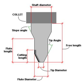
The **Free length** is the length of the part of the tool below the collet. So this is not the total length of the cutter. The free length is not constant, as it depends on how far you insert the cutter in the collet. DeskProto uses this
