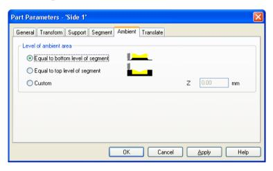
As DeskProto always creates toolpaths for a rectangular area, and as most prototypes do not have a rectangular geometry, some area will be present without geometry. This is called the ambient area. Or in other words, the area where no geometry is present, seen from the top. Here you can specify the level (or height) at which the ambient area should be milled.
