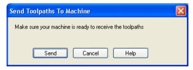
A dialog as shown above will be displayed to ask you if the machine is ready. After pressing Send DeskProto will start sending.
