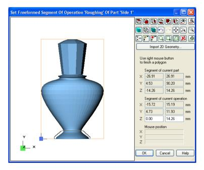
The Set Freeformed Segment dialog shows a new drawing of your part, and allows you to draw any closed freeform contour line in the Top view of your Part. The orange rectangle shows the Part segment: the freeformed segment needs to be completely inside this rectangle.
