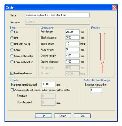
The **Name** is the name that will appear in any DeskProto dialog for selecting a cutter. It needs not be the same as the filename: use a name that clearly indicates which cutter you mean. Do show whether you mean radius or diameter for any number in this Name (you will forget if 'Ball6' means R6 or D6). Each cutter must have a unique name.
