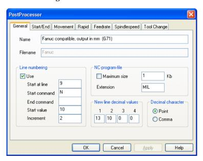
The **Name** is the name that will appear in any DeskProto dialog for selecting a postprocessor. It needs not be the same as the filename: use a name that clearly indicates which postprocessor you mean. Each postprocessor must have a unique name.
