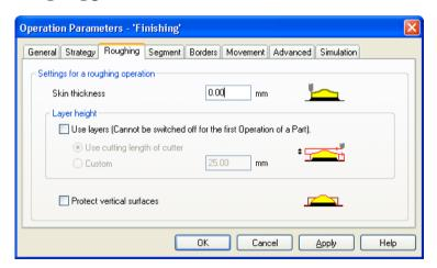
Roughing stands for quickly getting rid of most of the material without milling very precisely. So after an roughing operation you always need a second operation which machines the same area accurately: the finishing operation. In DeskProto you can use an operation either for roughing or for finishing, so if you need both you will have to **Add** an operation in the General Part parameters.
