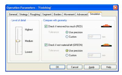
A **Simulation** is a drawing on screen that shows you what the resulting part will be. This can be used to check things like the resulting surface smoothness, error movements (if possible) that damage the part, rest-material where the cutter cannot reach, etc. In this dialog you can only set the simulation parameters. You can calculate a simulation by using the Calculate Simulation command in the Create menu. You can also switch the simulation on and off in the Subjects in view Dialog.
