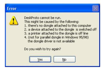
When no DeskProto Dongle can be found the above error message is displayed. Below you will find some suggestions in case of Dongle problems. The list has three sections: General, Parallel and USB.
