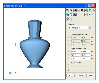
The dialog shows a new drawing of your part, with a rectangle that indicates the support block that you are editing. The buttons on the right can be used to influence the drawing. Eleven of these are standard DeskProto buttons of which the use is known, and that need no explanation here. Note that mouse rotation is not present: this dialog only used the six main views.
