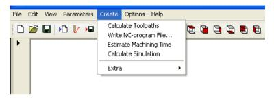
These options control all actions for calculating and saving NC toolpaths. Note the submenu called Extra which offers some extra options. As these are very specific and not important for most users these commands have been "hidden" in a submenu.
