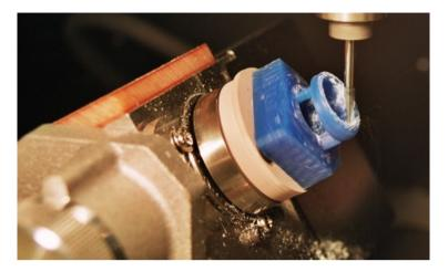
In the bottom-left corner of this picture you can see a rotation knob: after unlocking the rotation mechanism you can use this knob to manually tilt the complete rotation axis (A-axis) unit. This machine supports locking on fixed intervals of 15 degrees.
