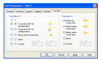
As a final part parameter DeskProto will apply an (automatic) translation to your geometry. Although you can see translation as a form of transformation, it's not placed in the transformation tab page. In DeskProto the translation is applied after all actual calculations, just before saving the toolpaths to an NC-program.
