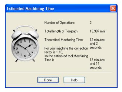
Theoretically speaking the calculation is very easy: DeskProto knows both the length of the toolpath and the feedrate (machining speed), so length divided by feedrate results in a theoretical machining time. However the real machining time is influenced by the answers to questions like:
