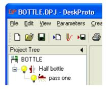
You can imagine the tree-like structure of a project, which is displayed in the Project Tree at the left side of the DeskProto screen: see the figure above. The basic Project consists of one (nameless) Part and one (nameless) Operation. In the illustration the project is called Bottle, containing one Part called 'Half bottle' and one operation called 'operation one'.
