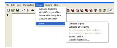
These Extra commands also are options for calculating and saving NC toolpaths. As these Extra commands are very specific and not important for most users these commands have been "hidden" in a submenu.
